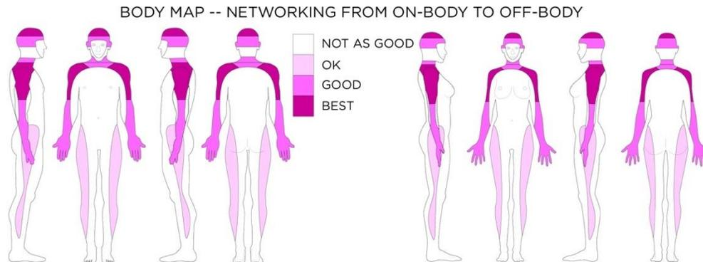
*BODY MAP 10 – Networking from the Body Map - This body map shows the areas on the body where a network antenna (to communicate to the fixed off-body wireless frequencies) could be placed to have the least chance of signal interference by the mass of the body.*
