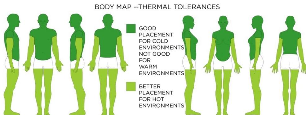
*BODY MAP 5 – Zones of Thermal Tolerance - This body map shows where to place wearable technology (which adds heat through operation and added bulk and material). This map focuses on a device’s tendency to raise overall body temperature; however, tissue on the body can burn at any location if exposed to enough heat over time.*
