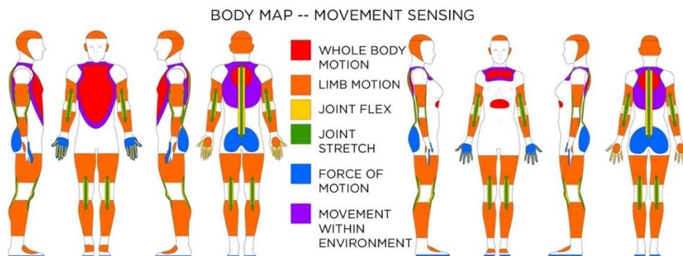
*BODY MAP 4 – Movement Sensor Placement - For sensing whole body motion, and limb motion, accelerometers, gyroscopes, and magnetometers can be used at locations indicated. For sensing joint movement, flex or stretch sensors can be used at locations indicated. Force can explain the impact of movement. If trying to capture movement within an environment, magnetometers (for direction) and barometric pressure sensors (for elevation change) may be used.*
